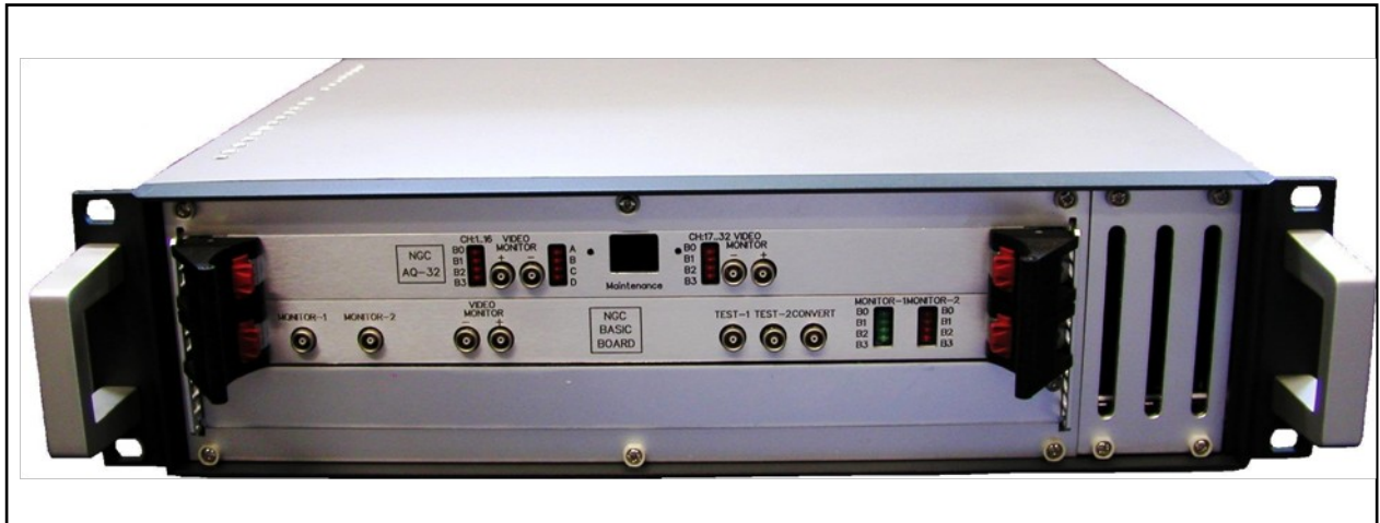
Figure 5 NGC Two-Slot System - Front side view
