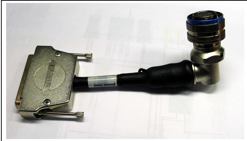
Figure 23. CCD cryostat video cable
