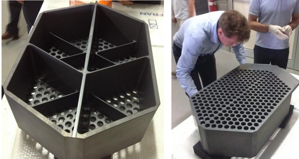
Figure 9. SiC Reference Body of the M4 demonstration Prototype. On the left one can see the back side and the variation of rib thickness due to manufacturing uncertainties. On the right side, the front face of the reference body.
