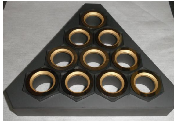
Figure 3. Silicon Carbide prototype with glass tiles bonded on it. One side of the capacitive sensor armatures is coated on each tile.
