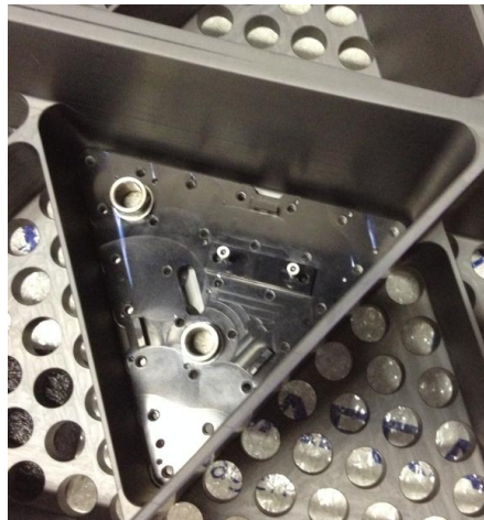
Figure 9. SiC Reference Body of the M4 demonstration Prototype. On the left one can see the back side and the variation of rib thickness due to manufacturing uncertainties. On the right side, the front face of the reference body.
