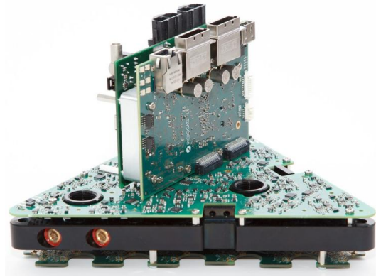
Figure 7. Standard brick of 28 actuators. The capacitive sensor board is located at the bottom of the brick; the voice coil driver board is on the upper face of the brick while the control and power supply boards are located on each side of the vertical heat sink.
