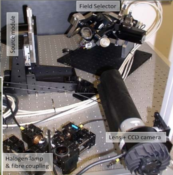
Above: the GALACSI Field Selector on a test setup: the Field Selector, source module, Lamp housing/fibre injection and motor controllers are in use.
