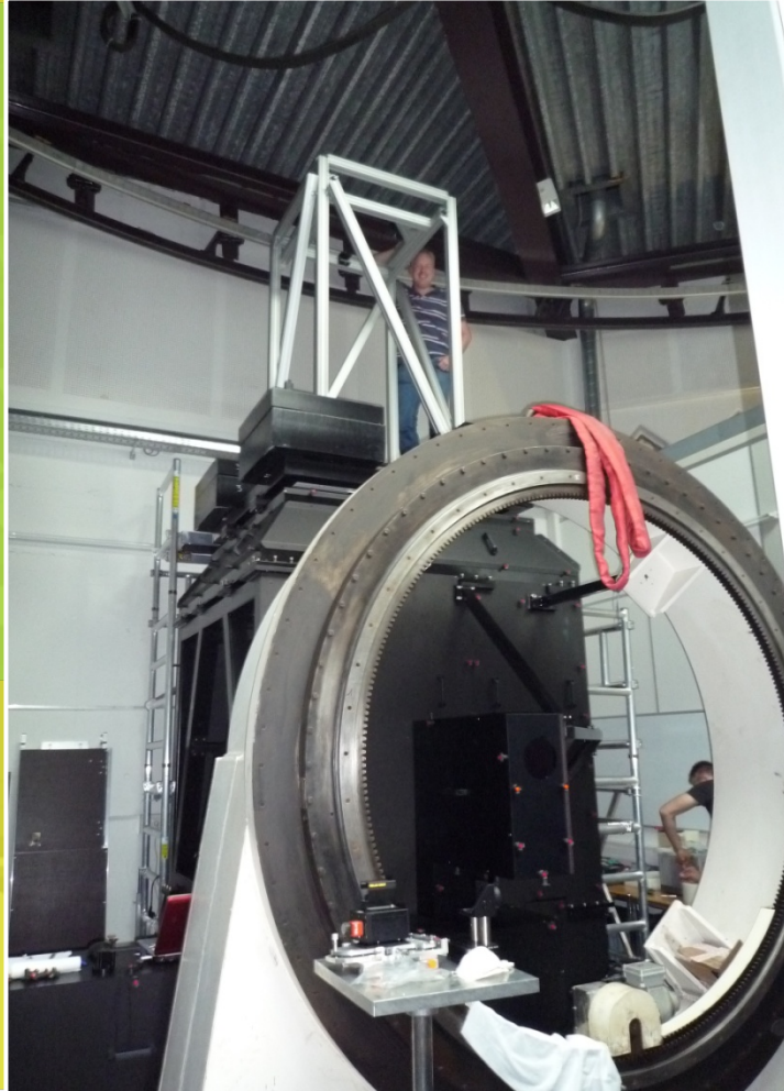
Right: the whole structure assembled (June 2011): DSM tower, Shack-Hartmann tower and adaptor ring. The total height is more than 5 m.
