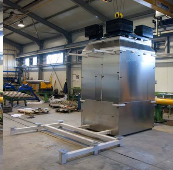
Above: full assembling of the ASSIST main structure mechanics at Boseenkool (NL) (February 2011). Left: the tower before enclosure. Right: with enclosure. On top of the tower the dummy loads simulating the DSM weight are visible.
