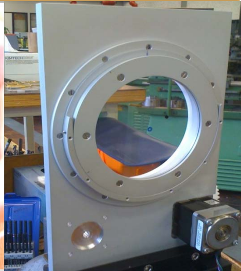
Below: the frame allowing Phase Screen exchange and rotation. This is part of the Star Simulator and Turbulence Generator module (SSTG). The Phase Screens allow to simulate a seeing and turbulence profile including coherence.
