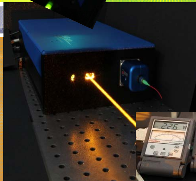
SHG prototype. Above: open top view. Below: 22.6 W output power @589 nm have been demonstrated.
