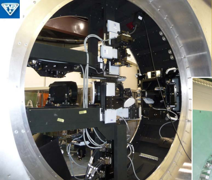
Above: GALACSI almost completely assembled, during testing at ESO. Except the LGS wavefront measuring path, GALACSI is already equipped with all the optics.
