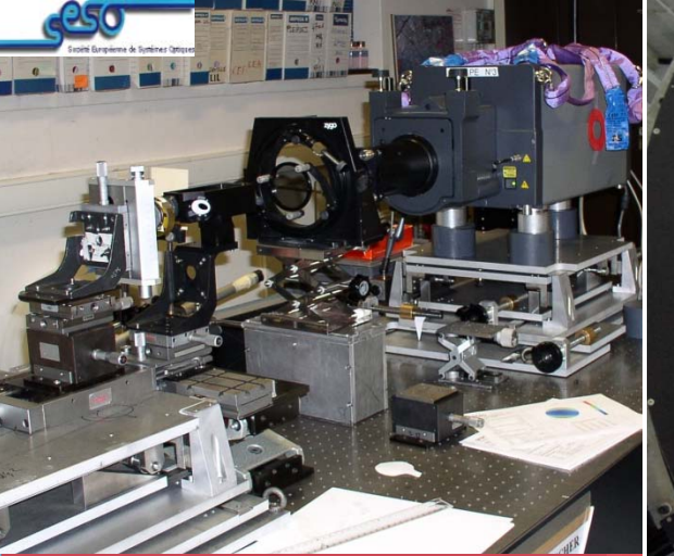
Below: one of the LGS pick-up arm mounted on its Physik-Instrumente translator, installed inside the GRAAL rotating flange at NTE..
