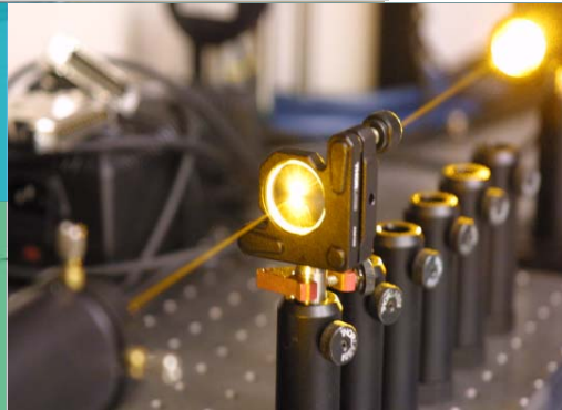
Above: testing of coating samples at focus under high laser power illumination (March 2010)
