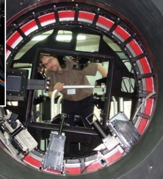
Above: from bottom left, clockwise: TT unit, LGS calibration assembly, MCM lens (February 2011). Below: during assembly of the the rotating frame at NTE (September 2010)
