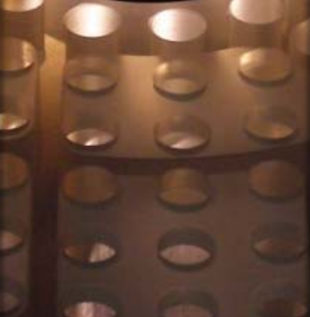
Final inspection of the reference body at SESO. The unit is ready for the metal coating deposition on the internal sides of the holes, for the capacitive sensor.
