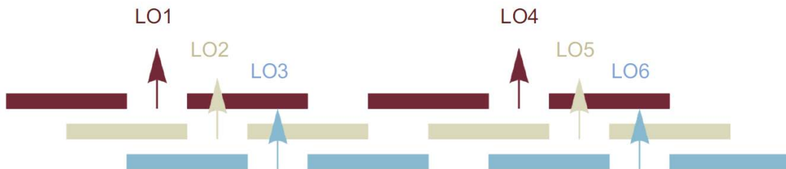
Figure 21: IF coverage 4-20 GHz 2SB: 6 tunings for 88GHz double coverage
