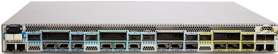
Figure 5: COTS 1.6 Tb/s chassis capable of hosting 400 GbE modules
